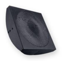
Grid Spot Attachment is designed to fit directly over your flash unit's standard 7-inch reflector. This built-in grid reflector will take the 80° beam spread of your standard reflector down to a highly controllable 18° spread for a back or hair light
